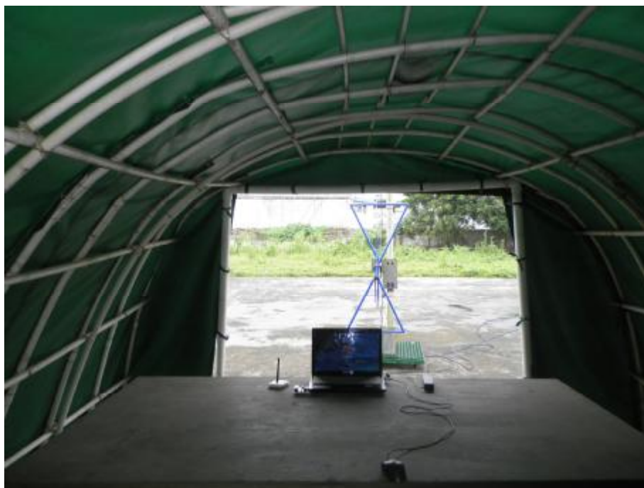
Radiated emission test view
