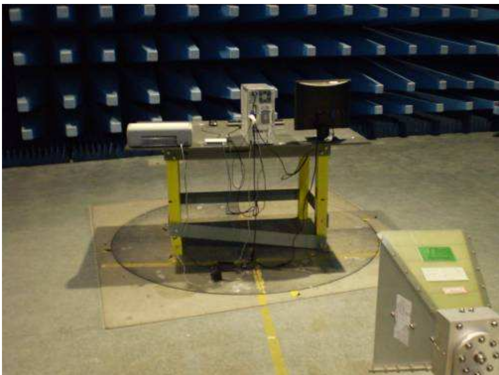
Radiated Spurious Emissions Test Setup (Above 1GHz)
