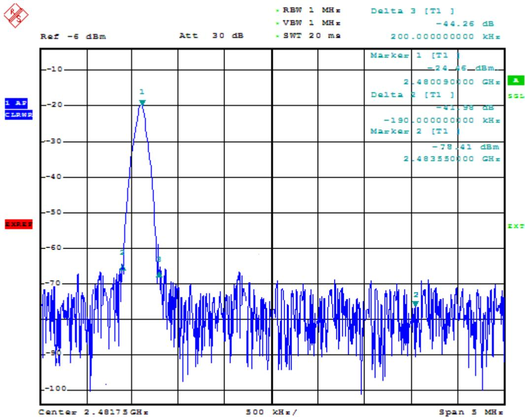
For band frequency 2.4835GHz, test level is -78.41dBmW,
