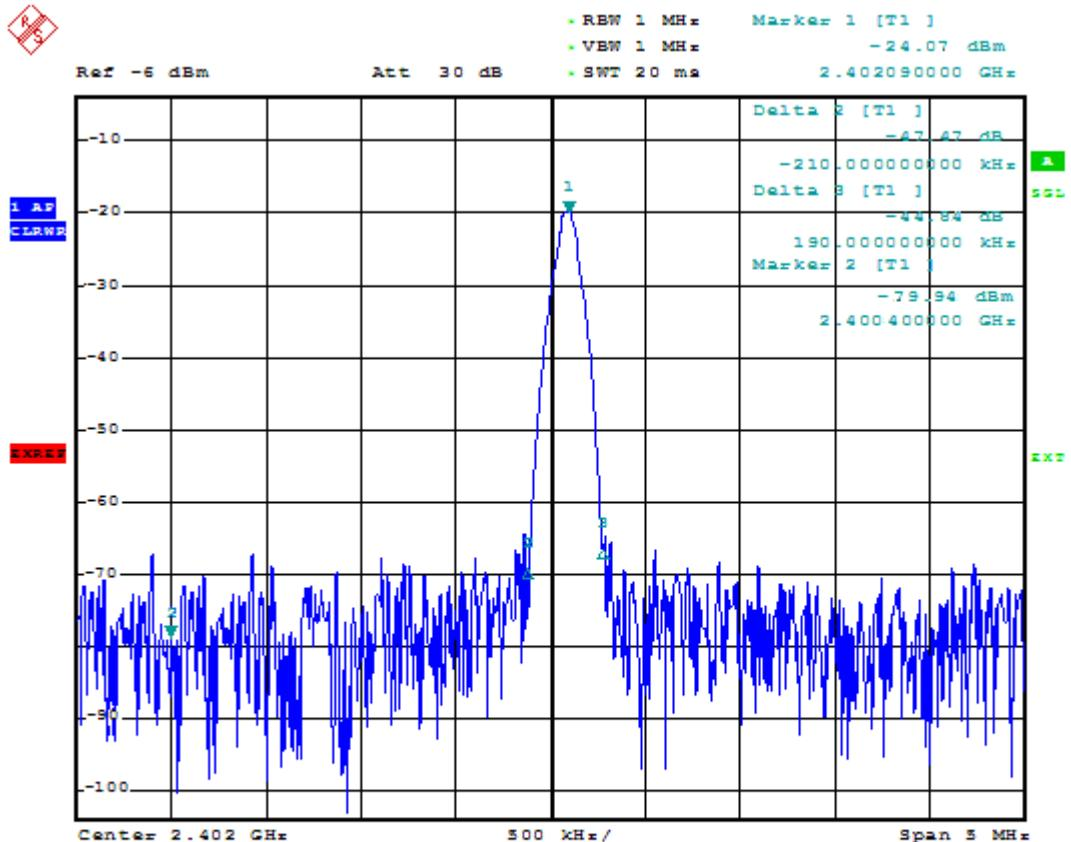
For band frequency 2.400GHz, test level is -79.94dBmW,
