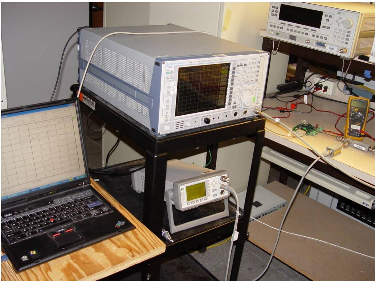
Radiated Spurious Emissions – Test Configuration
