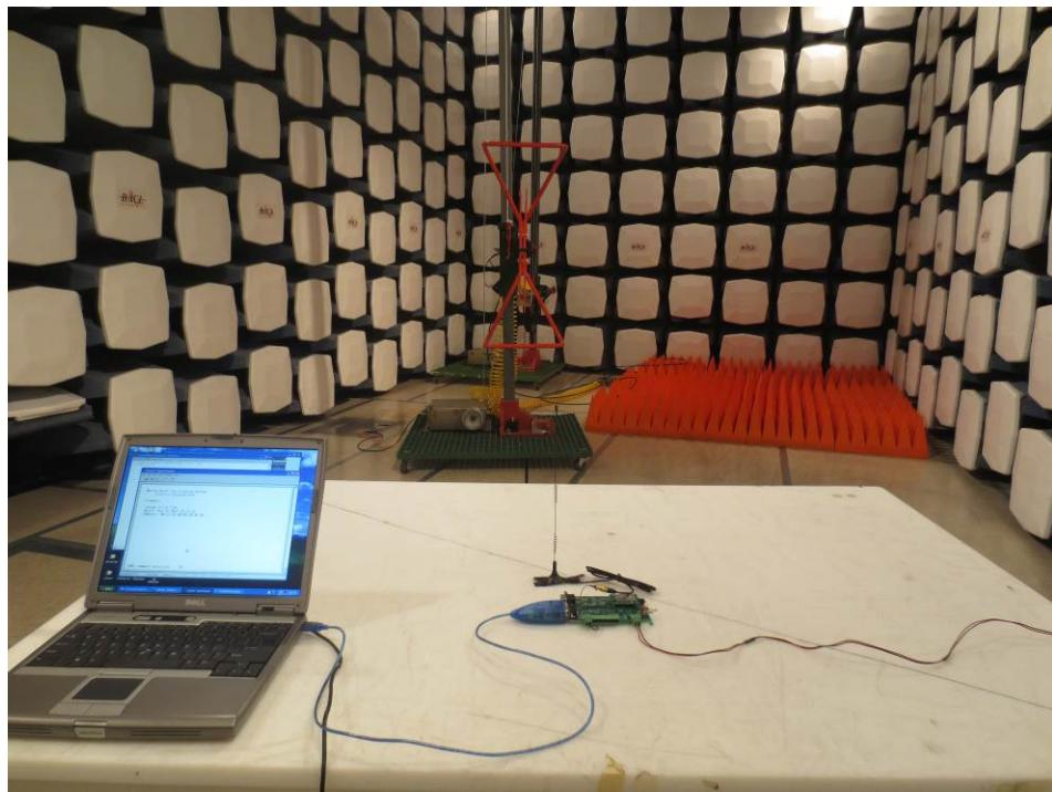
**12.7 Radiated Emission below 1 GHz Rear View – 14.5 dBi Antenna**
