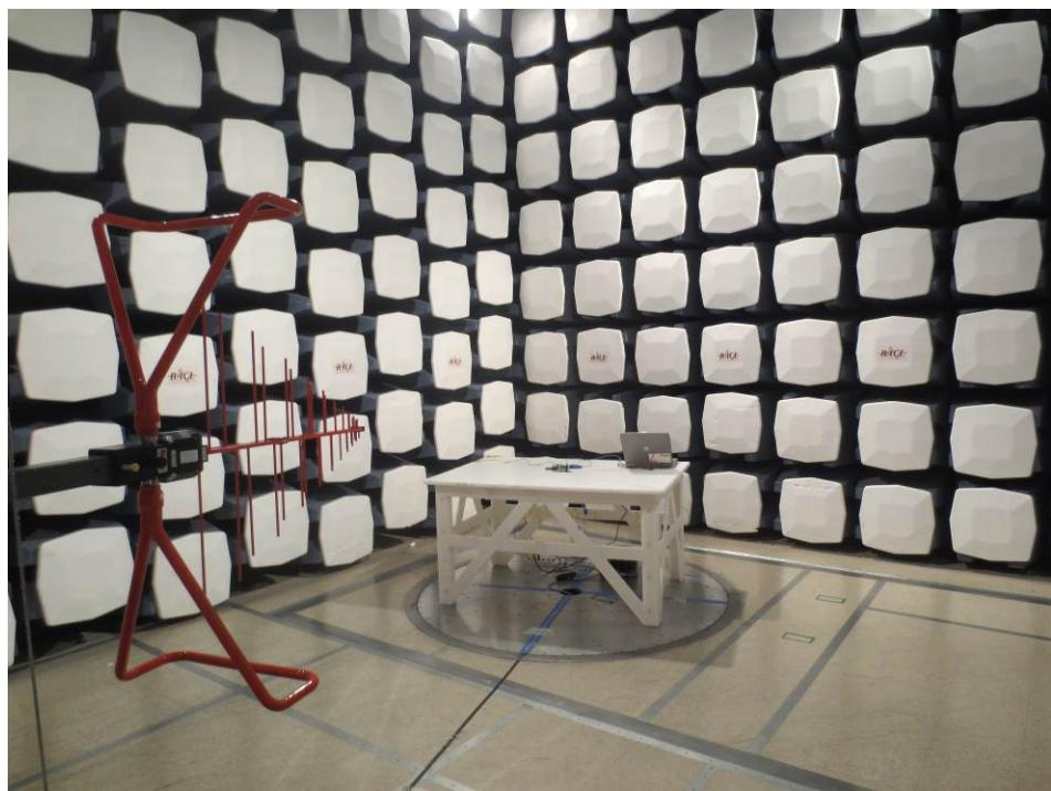
**12.6 Radiated Emission below 1 GHz Rear View – 7 dBi Antenna**
