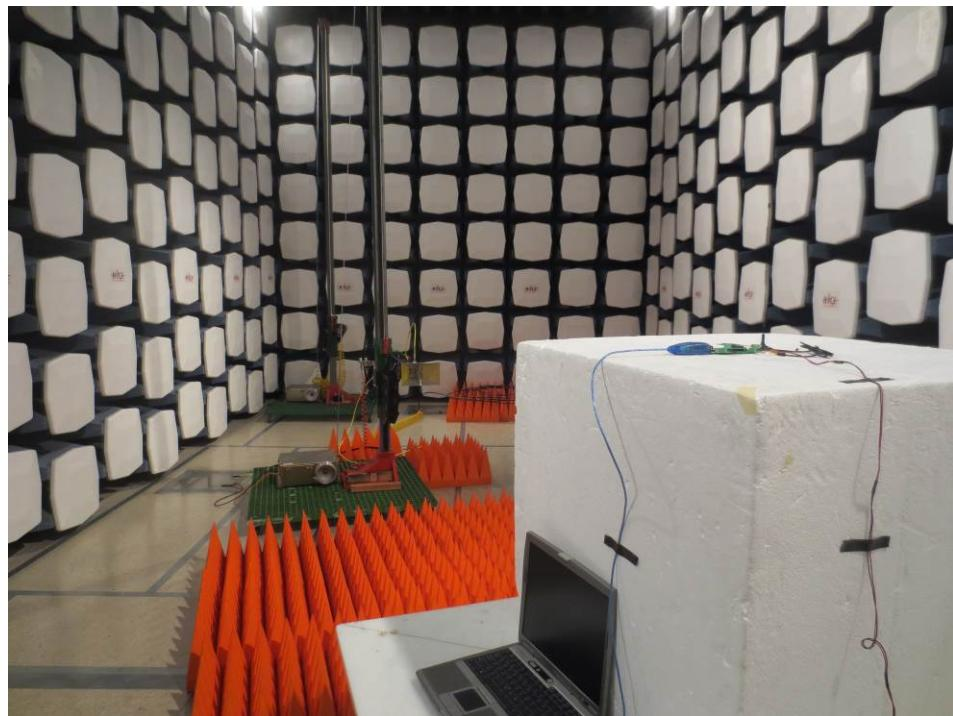
**12.13 Radiated Emission above 1 GHz Front View – 14.5 dBi Antenna**
