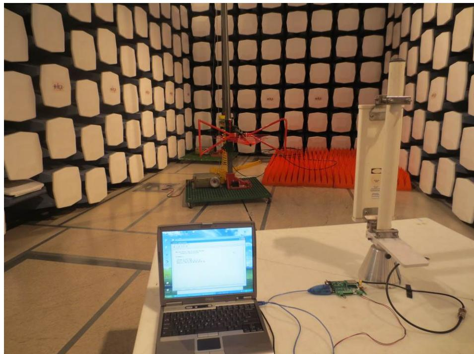
**12.9 Radiated Emission above 1 GHz Front View – 3.5 dBi Antenna**
