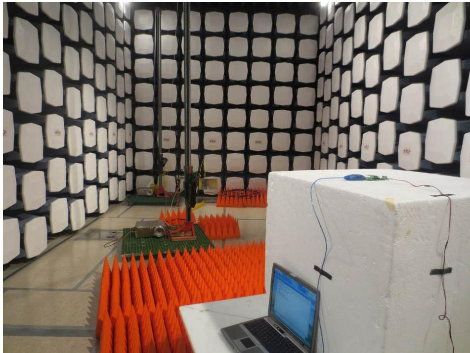
**12.11 Radiated Emission above 1 GHz Front View – 7 dBi Antenna**
