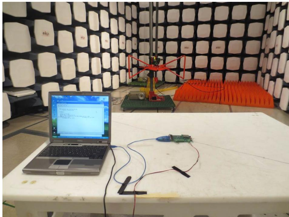
**12.5 Radiated Emission below 1 GHz Front View – 7 dBi Antenna**
