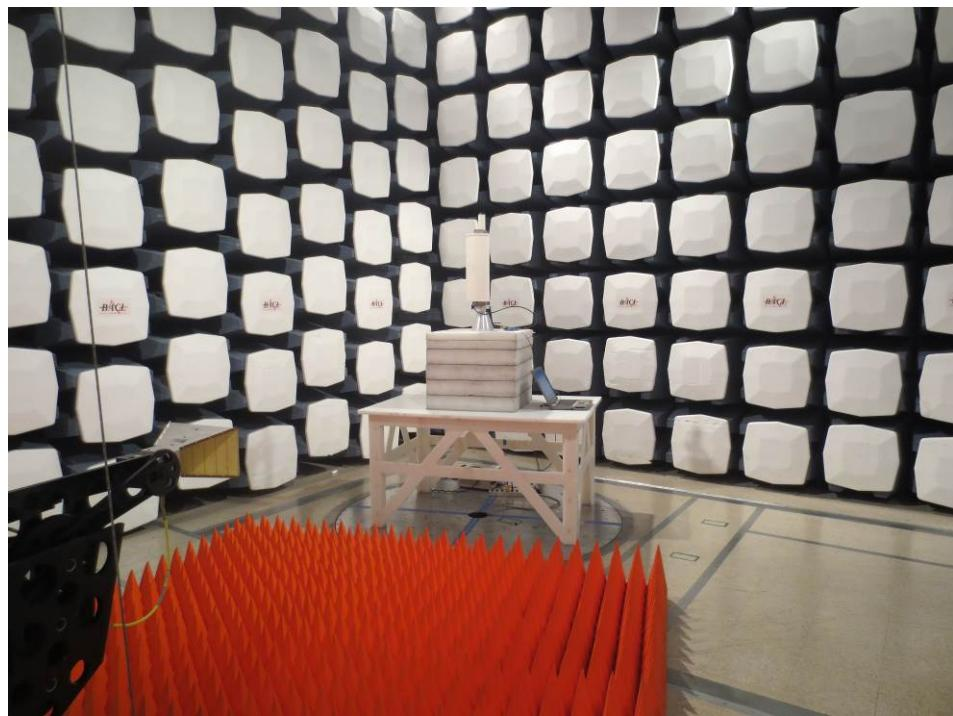
**12.14 Radiated Emission above 1 GHz Rear View – 14.5 dBi Antenna**
