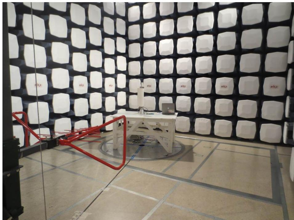
**12.8 Radiated Emission below 1 GHz Rear View – 14.5 dBi Antenna**
