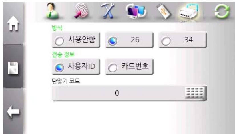
The “Type” field defines the usage of wiegand out lines. When enabled, 26-bit and 34-bit formats are supported.
