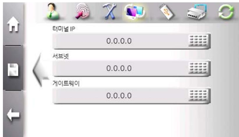
If DHCP is disabled, network configuration needs to be set manually. Network configuration consists of terminal IP, subnet mask and gateway IP. Please contact IT manager of office to get available setting.
