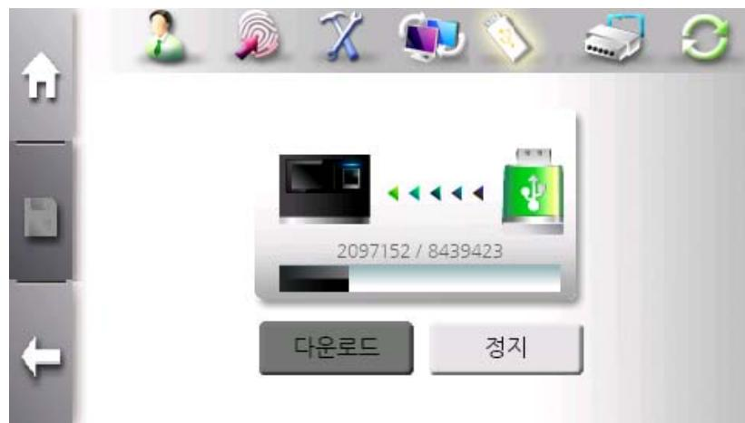
After inserting USB memory stick having SW300\_Cab.CAB file in root directory, click “Firmware Update” button. During copying, the progressing bar is displayed. If done, terminal will be rebooted.
