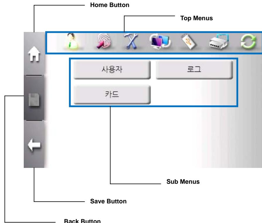
**“Home Button”** placed in left upper is used to quit current stage and go to initial display.
