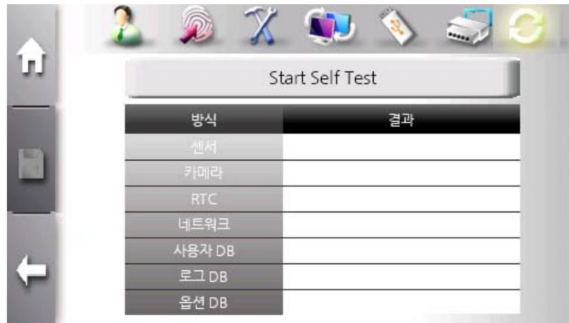
The diagnosis is started by clicking “Start Self Test” button. According to the result, “OK” or “Fail” is marked for each list.
