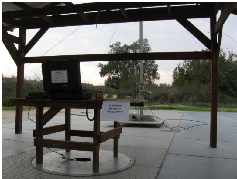
Figure 3. Radiated Emission test Setup
