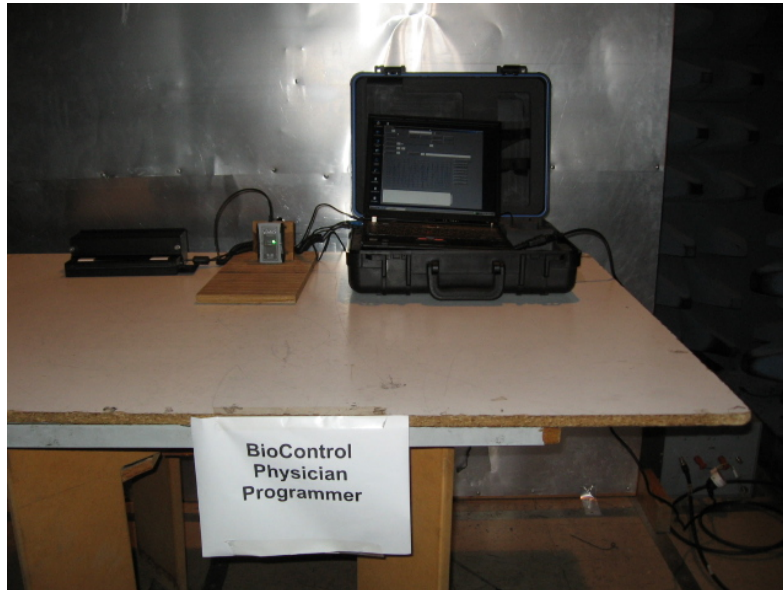
Figure 2. Conducted Emission test Setup
