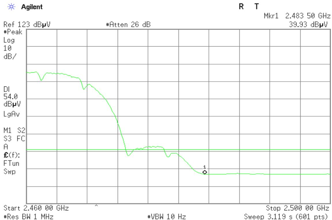
**Band Edges (IEEE 802.11g mode / CH Low)****Detector mode: Peak****Polarity: Vertical**
