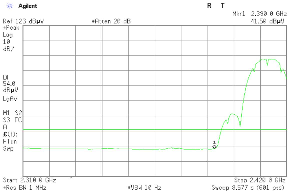
**Band Edges (IEEE 802.11b mode / CH High)****Detector mode: Peak****Polarity: Vertical**
