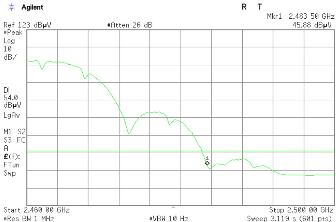
**Detector mode: Peak****Polarity: Horizontal**
