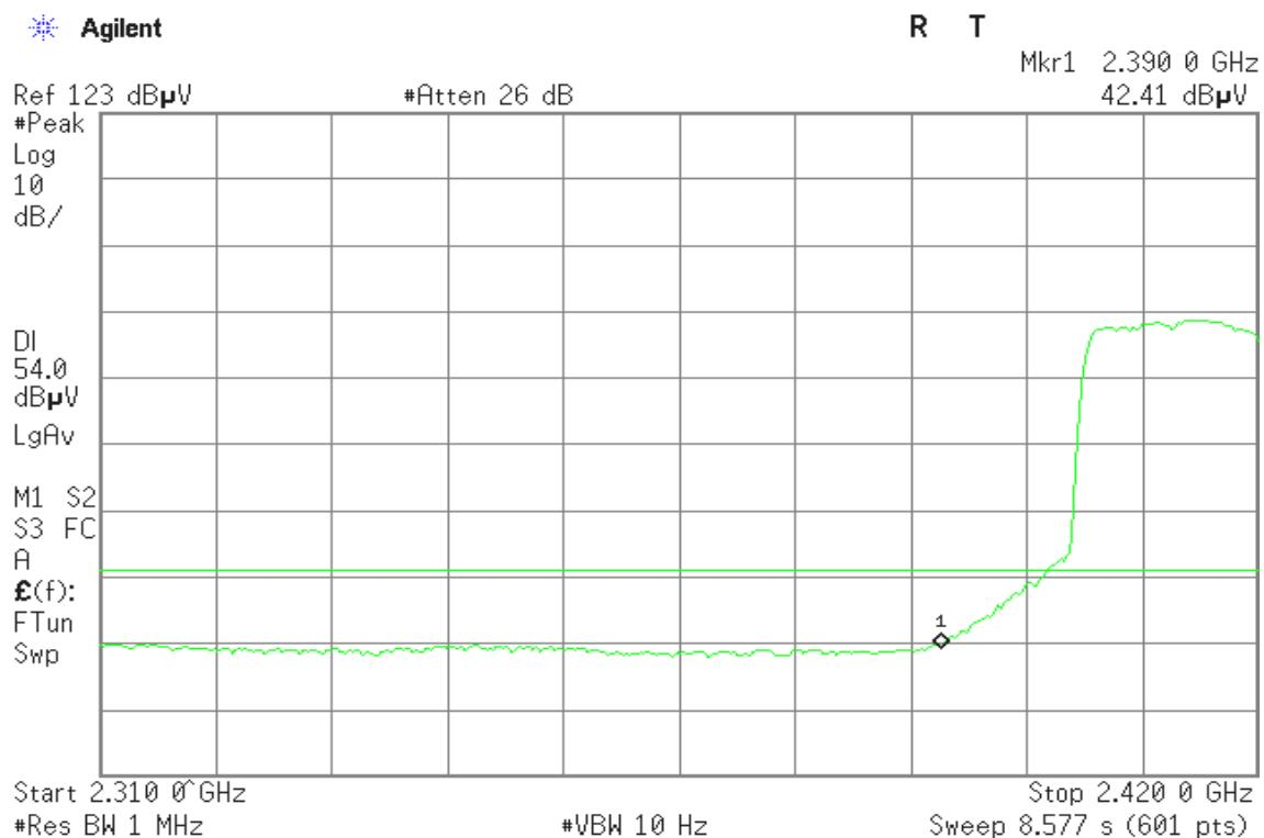
**Band Edges (IEEE 802.11g mode / CH High)****Detector mode: Peak****Polarity: Vertical**
