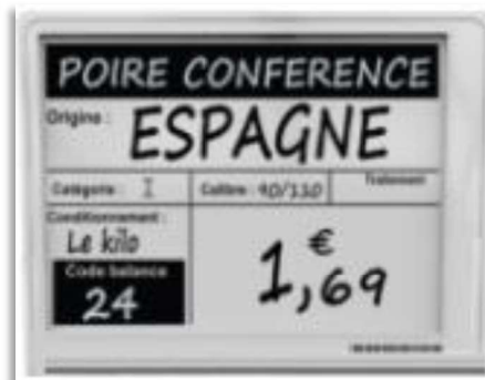
Figure 2: Electronic Shelf Label (ESL) or Tag
