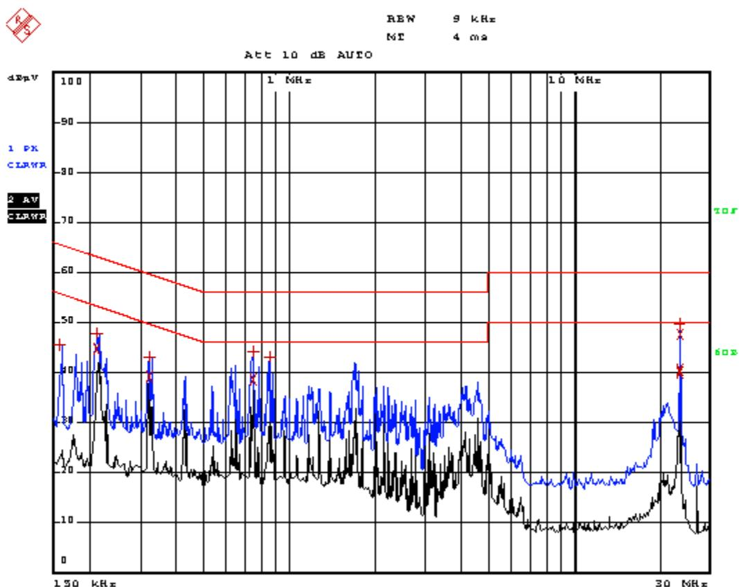
**Plot of Conducted Emissions Test Data***Conducted Disturbance**EUT: HDD MEDIA PLAYER**M/N: SO ROAD MOVIE**Operating Condition: Playing**Test Specification: L**Comment: AC 120V/60Hz Connect to TV*
