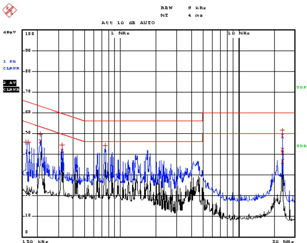
**Plot of Conducted Emissions Test Data***Conducted Disturbance**EUT: HDD MEDIA PLAYER**M/N: SO ROAD MOVIE**Operating Condition: Downloading**Test Specification: N**Comment: AC 120V/60Hz Connect to PC*
