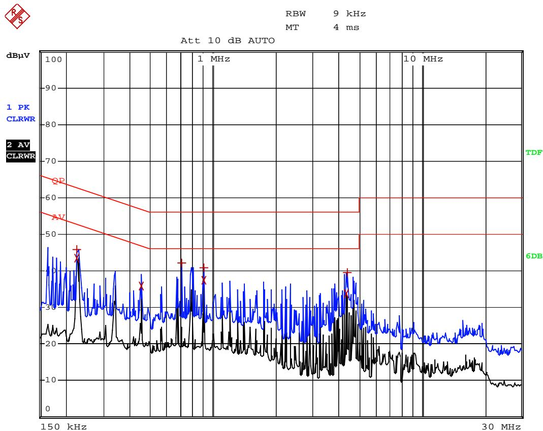
**Plot of Conducted Emissions Test Data***Conducted Disturbance**EUT: HDD MEDIA PLAYER**M/N: SO ROAD MOVIE**Operating Condition: Downloading**Test Specification: L**Comment: AC 120V/60Hz Connect to PC*
