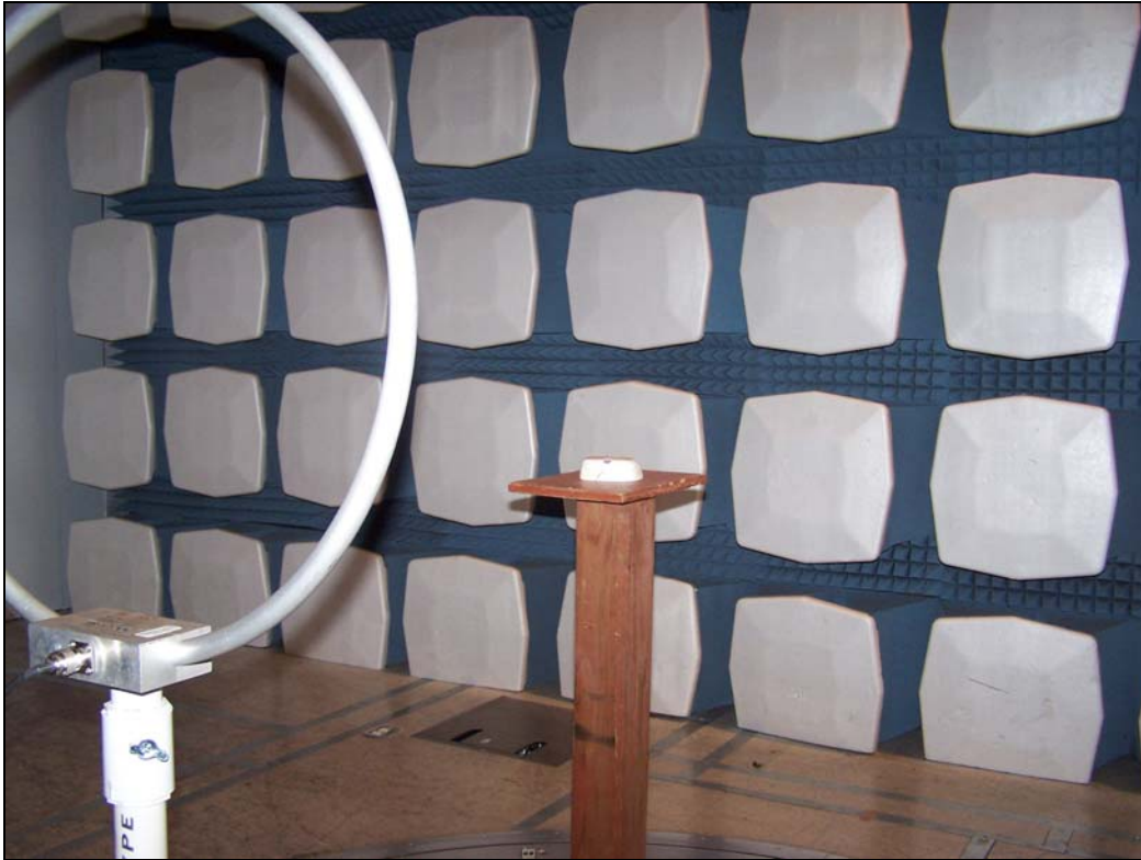
Photograph 2. Spurious Emissions Limits, Test Setup
