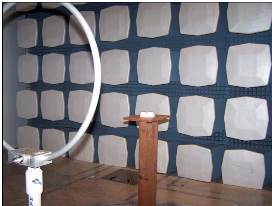
Photograph 6. Measurements below 30 MHz
