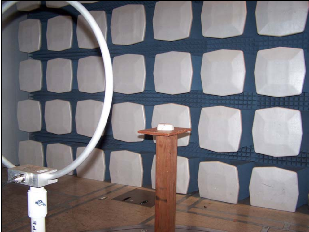
Photograph 3. Spurious Emissions Limits, Test Setup
