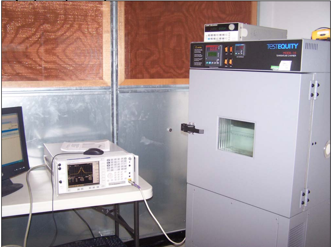
Photograph 7. Frequency Stability Test Setup
