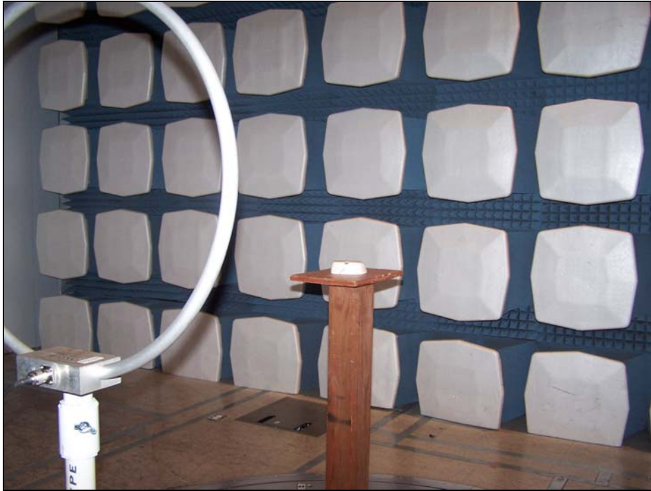
Photograph 1. 20 dB Bandwidth Test Setup
