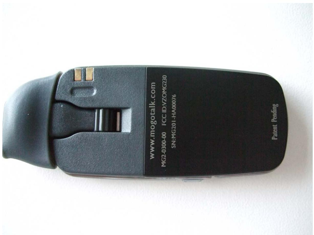
This label is printed by laser on the enclosure.
