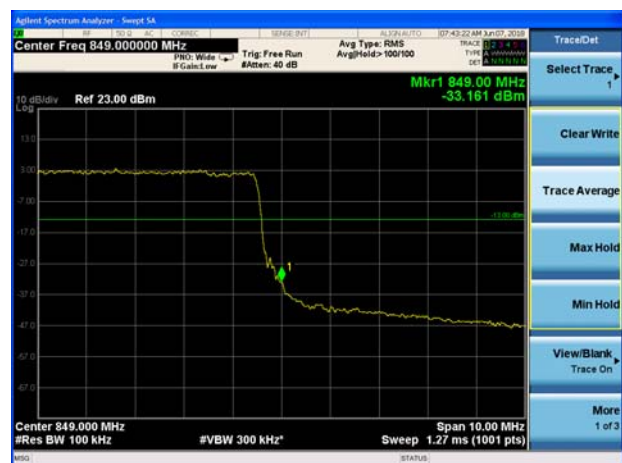
LTE Band 5 QPSK 10MHz CH-High 100%RB
