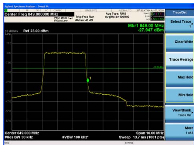
LTE Band 5 QPSK 5MHz CH-High 1RB
