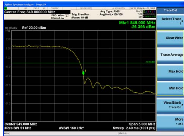
LTE Band 5 QPSK 1.4MHz CH-High 1RB
