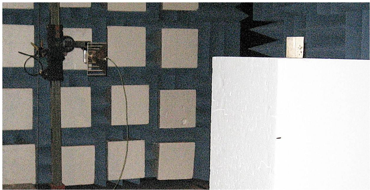
3. Test for Radiated Emissions with SAS-5, 9kHz to 30MHz
