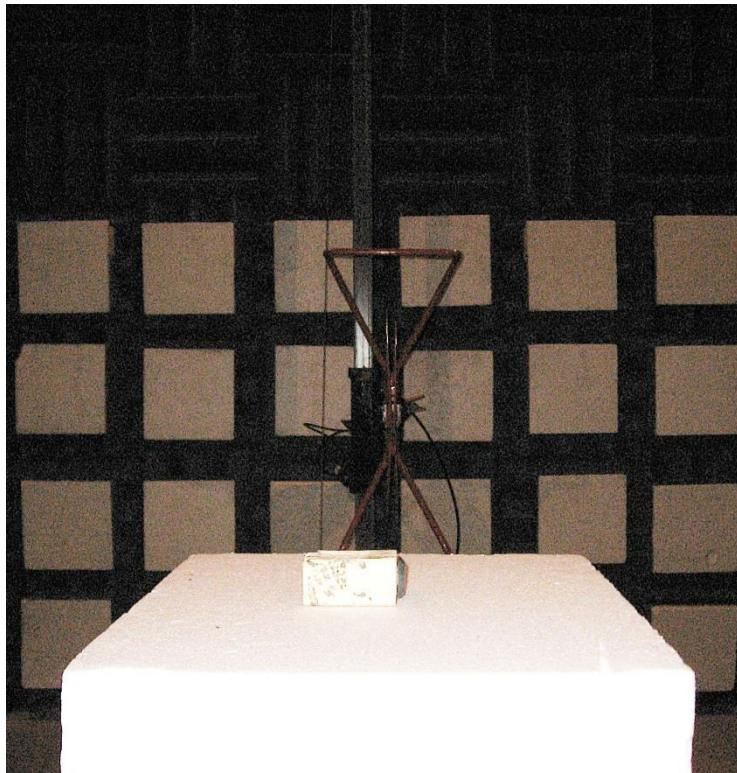
2. Test for Radiated Emissions with SAS-572, 1-6GHz
