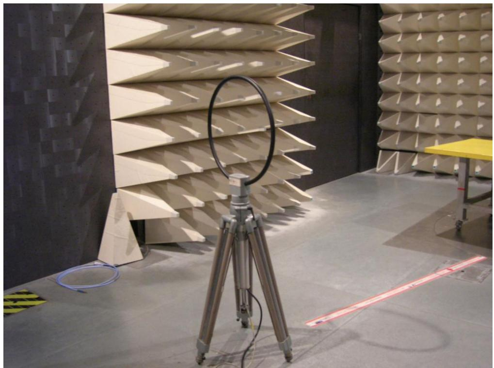
For radiated emissions 30MHz~1GHz
