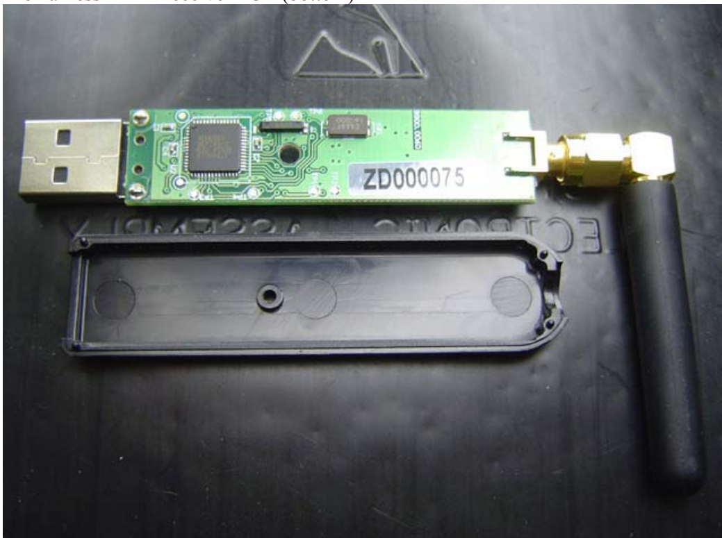
BioHarness™ RF Receiver PCB (bottom)
