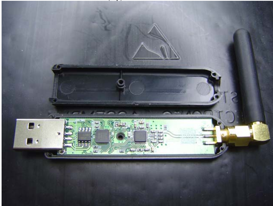
BioHarness™ RF Receiver PCB (top)
