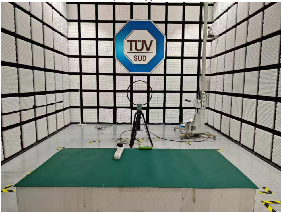
Radiated Emission Setup 9kHz ~ 30MHz
