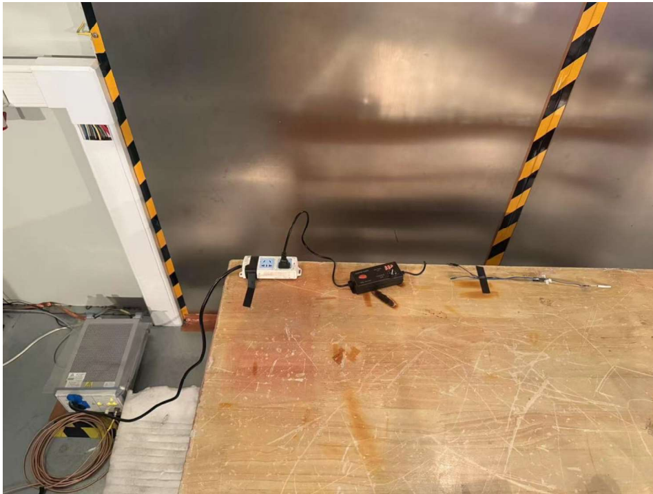
Test Set-up: Conducted emission 150KHz-30MHz
