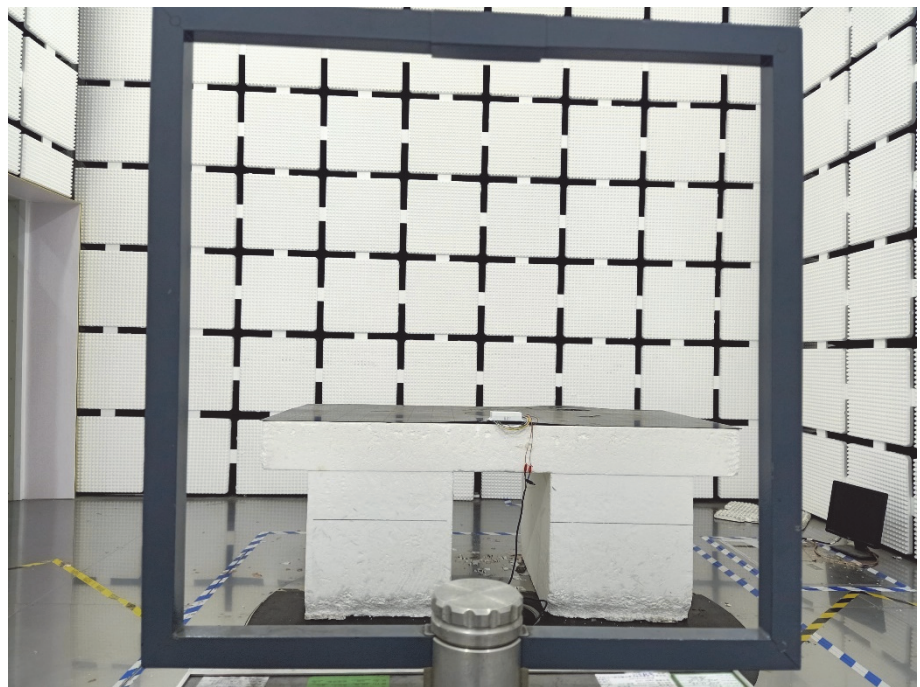
Radiation Emission Test Setup (Below 30MHz)
