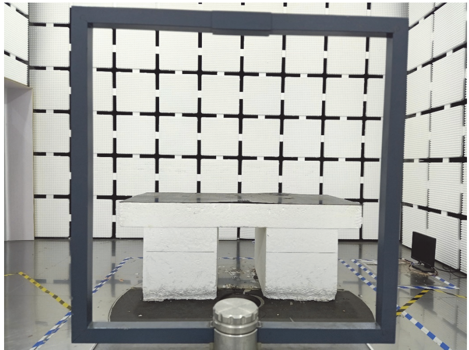
Radiation Emission Test Setup (Below 30MHz)
