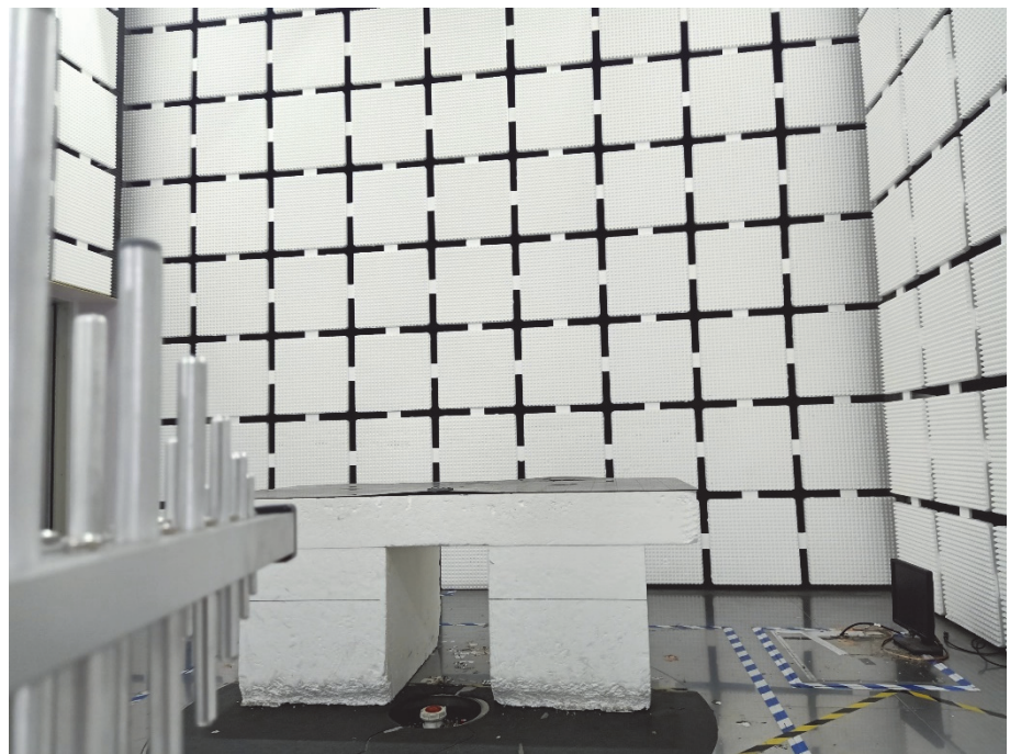
Radiation Emission Test Setup (30MHz to 1GHz)
