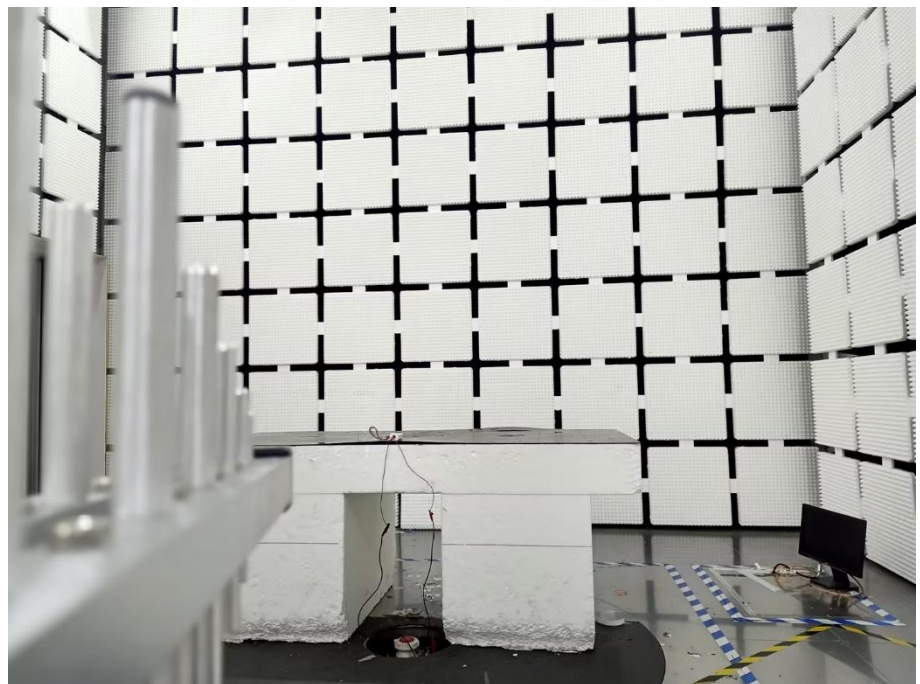
Radiation Emission Test Setup (30MHz to 1GHz)
