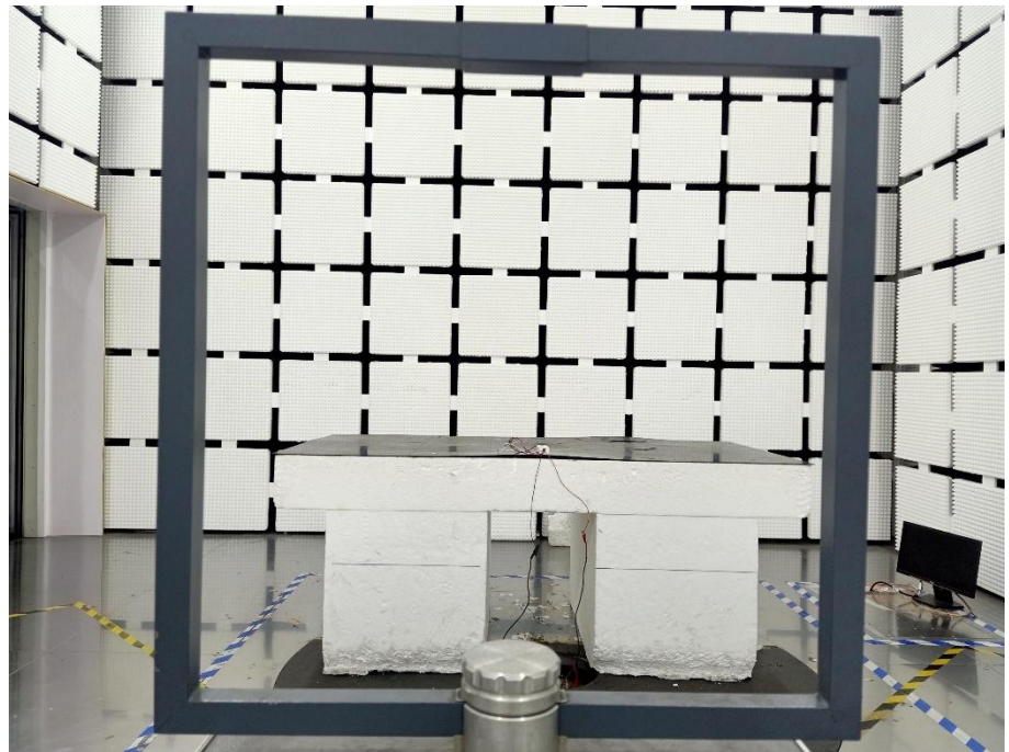
Radiation Emission Test Setup (Below 30MHz)
