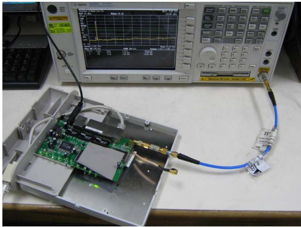
**POWERLINE CONDUCTED EMISSIONS MEASUREMENT SETUP**
