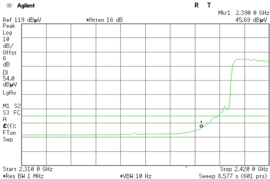
**Band Edges (IEEE 802.11g / CH High)****Detector mode: Peak****Polarity: Vertical**
