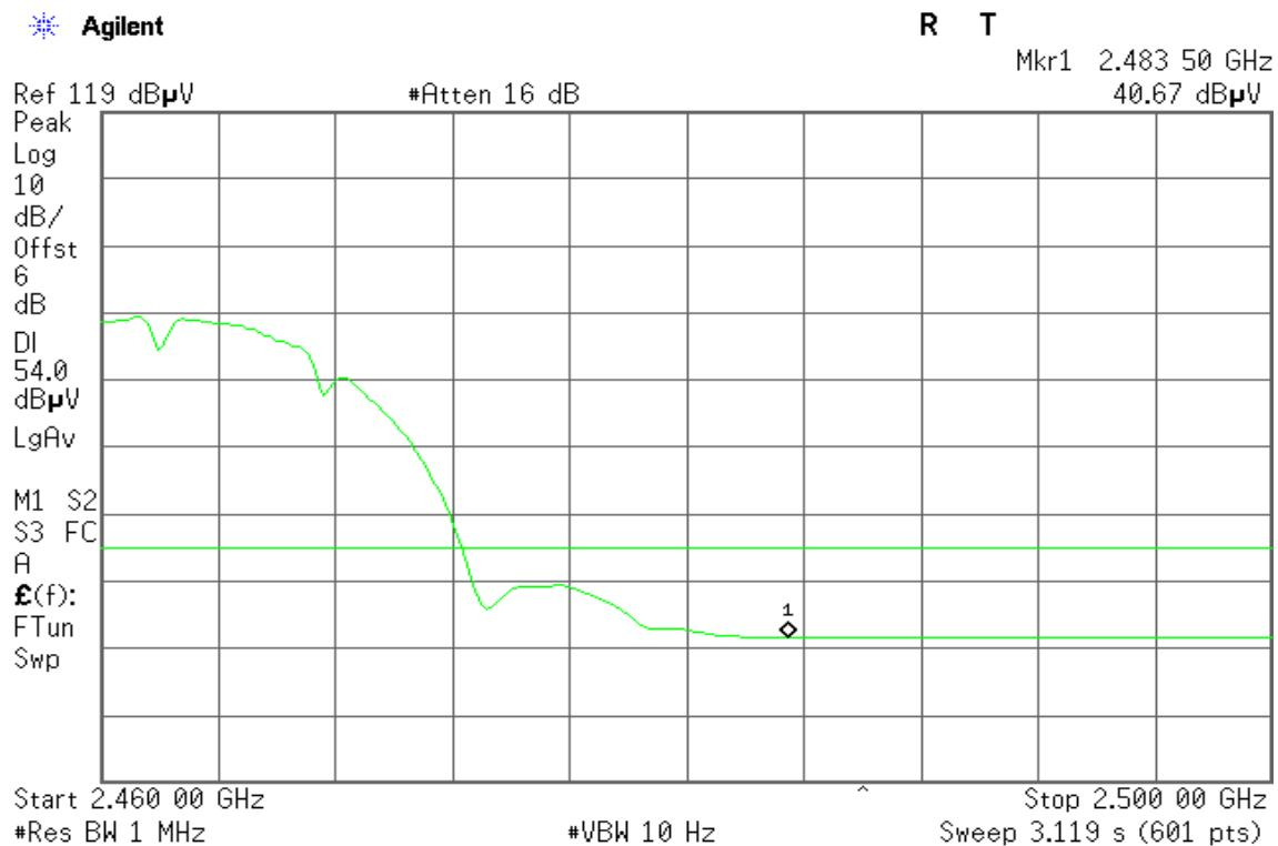
**Band Edges (IEEE 802.11g / CH Low)****Detector mode: Peak****Polarity: Vertical**
