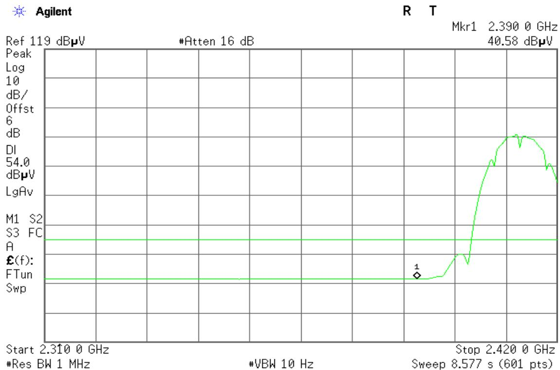
**Band Edges (IEEE 802.11b / CH High)****Detector mode: Peak****Polarity: Vertical**
