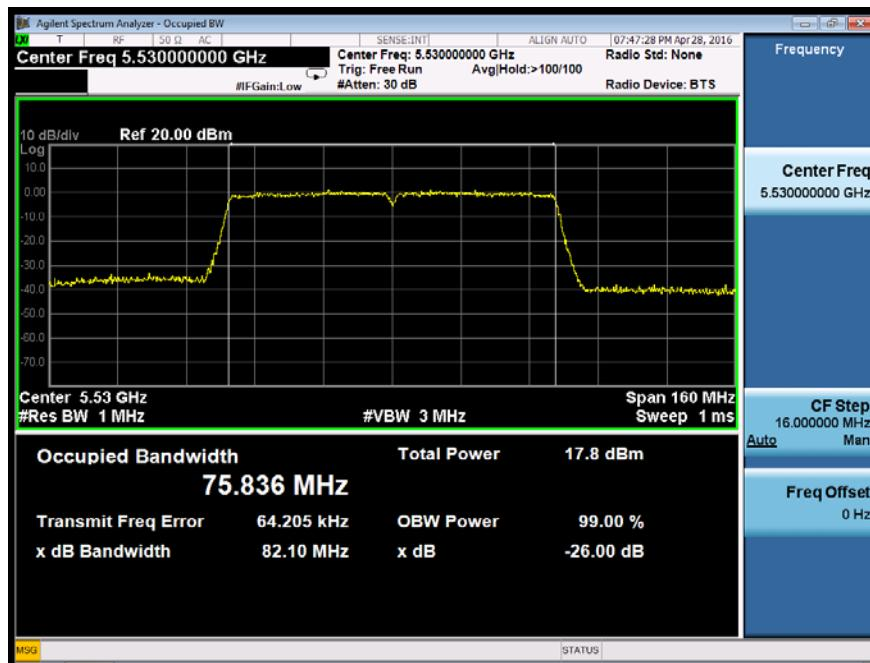
Emission Bandwidth&99% Occupied Bandwidth UNII Band II-C
