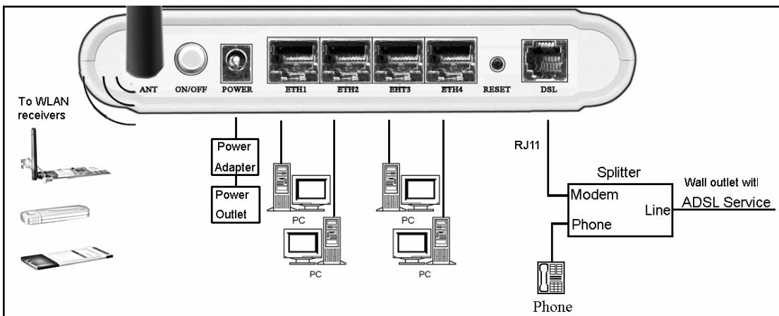
3. Connect the power cable to the PWR connector on **ROUTER**, then plug in the AC power adapter to the AC power outlet, and then press the on-off button.
