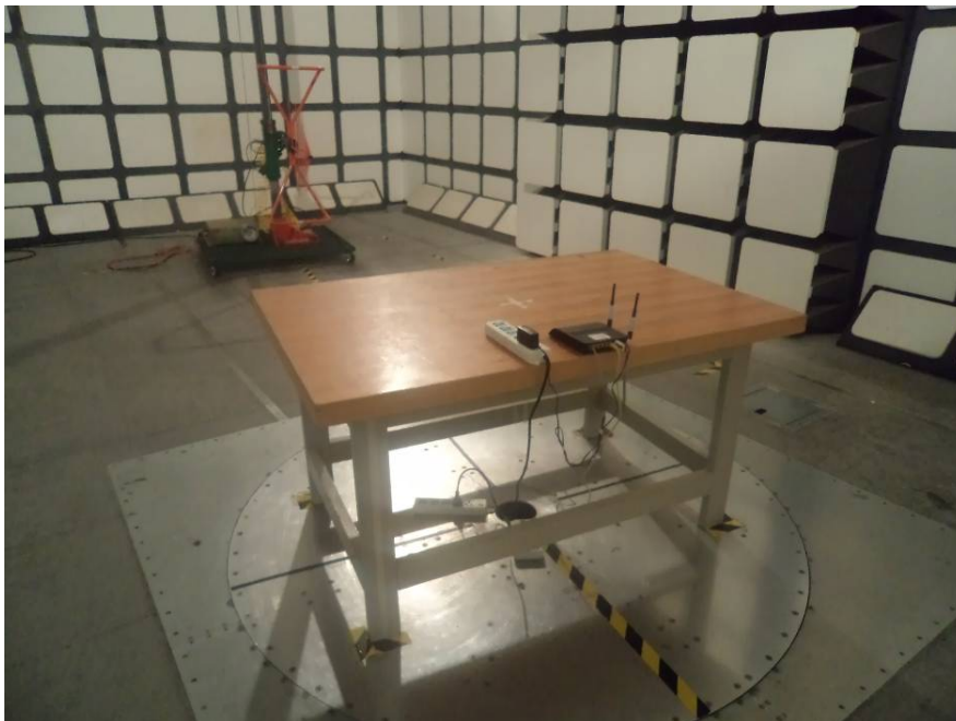
Spurious Radiated Emissions – Rear View (30 MHz - 1 GHz)
