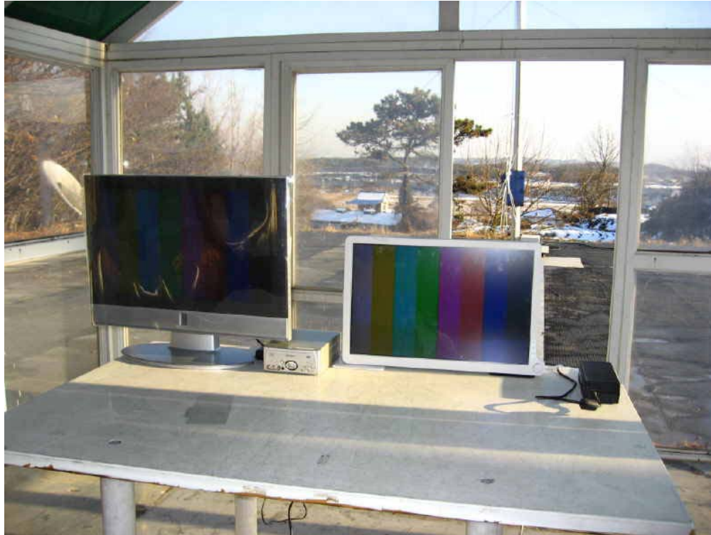
Figure 6. Photo of Radiated emission test setup
