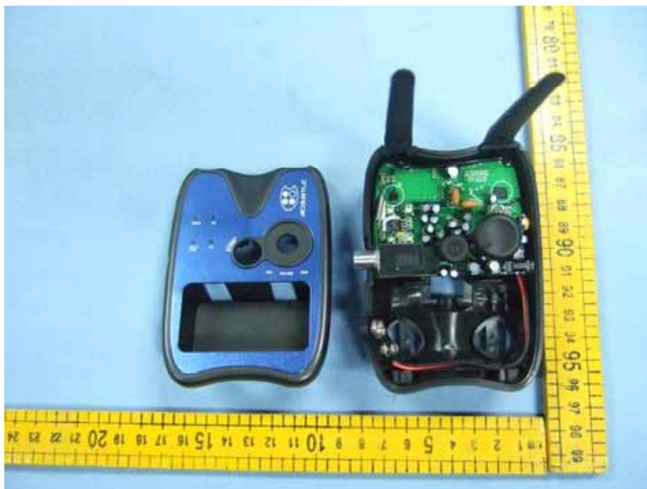
Figure 4 Receiver of the EUT-Inside View
