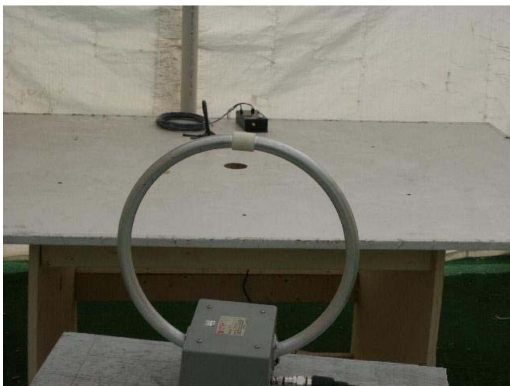
**Radiated Emissions Test Setup Photos (Stand Alone)**
