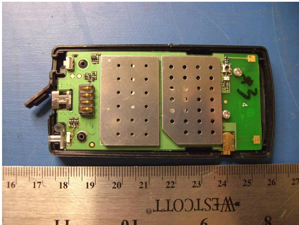
**EUT with Shield on – Front View**
