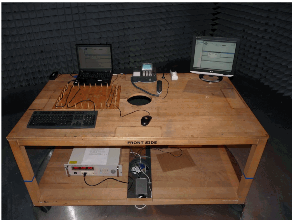
setup for the test radiated emissions
