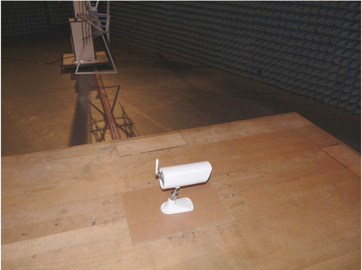
Photo 4: Test setup for output power radiated measurement
