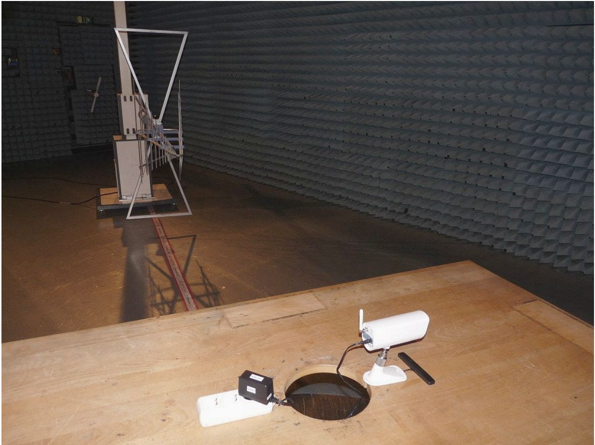
Photo 2: Test setup for radiated measurements, 30 MHz – 1 GHz
