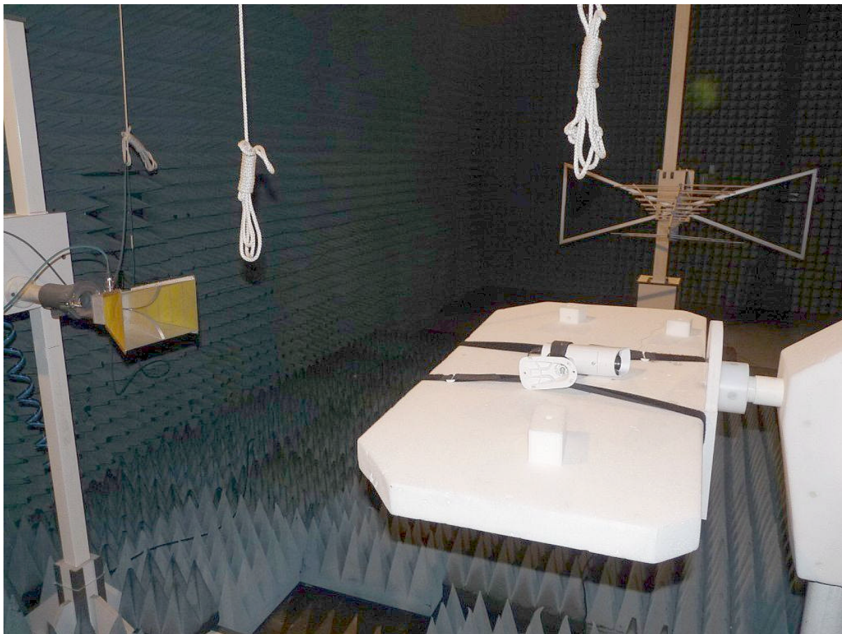
Photo 3: Test setup for radiated measurements, above 1 GHz
