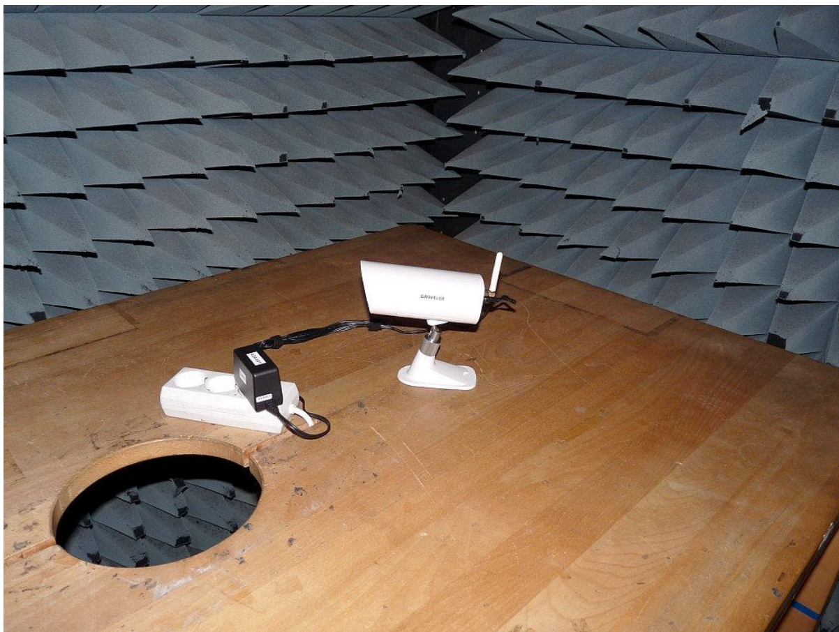
Photo 1: Test setup for radiated measurements, 9 kHz – 30 MHz
