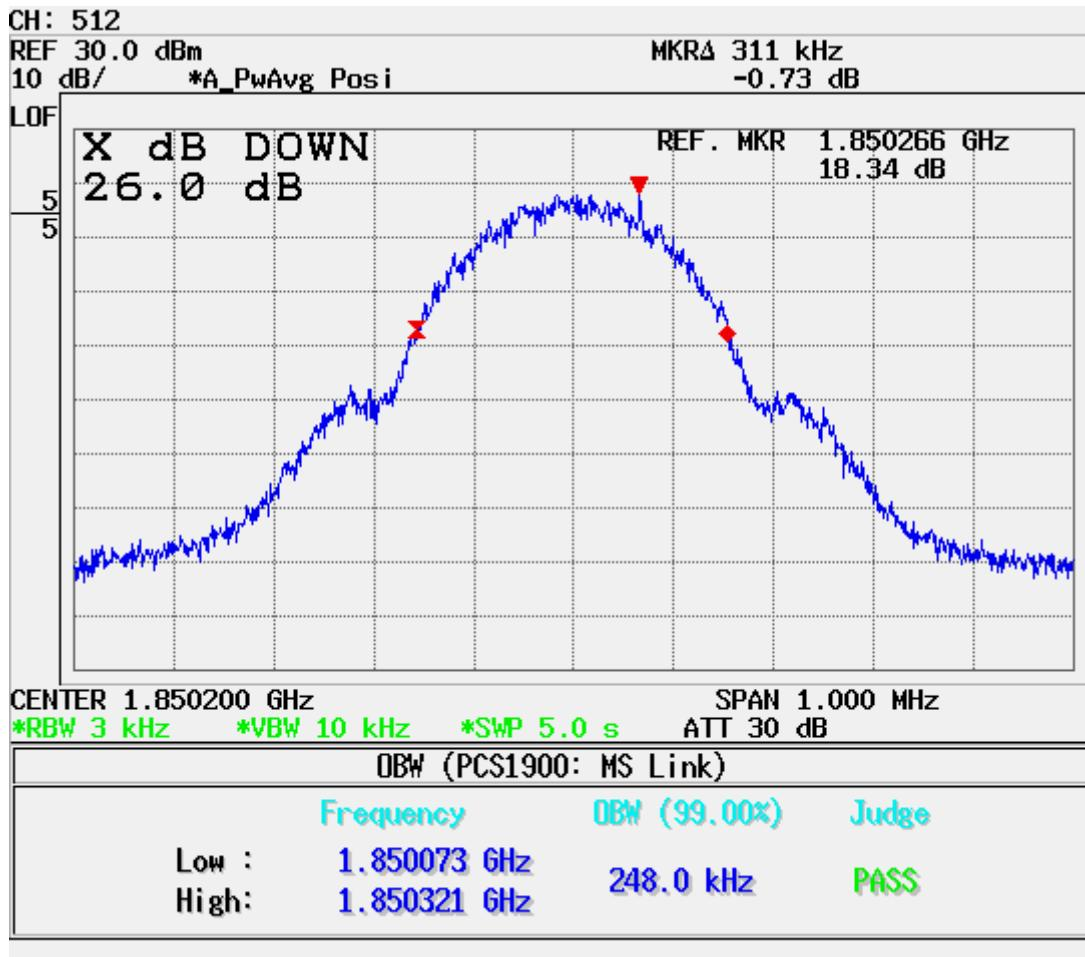
**■ Occupied Bandwidth – 26 dBc BW (KHz) (GSM1900 661 CH)**
