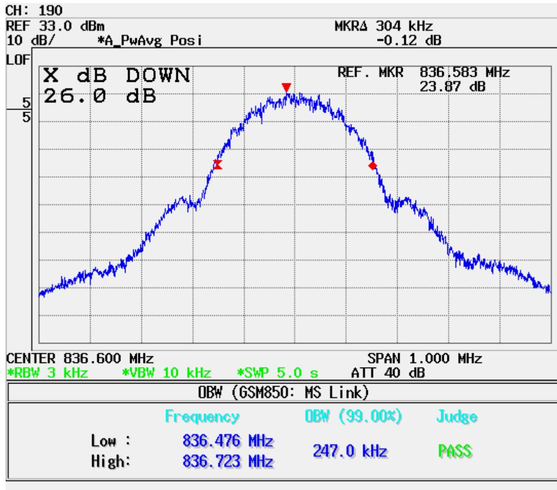
**■ Occupied Bandwidth – 26 dBc BW (KHz) (GSM850 251 CH)**
