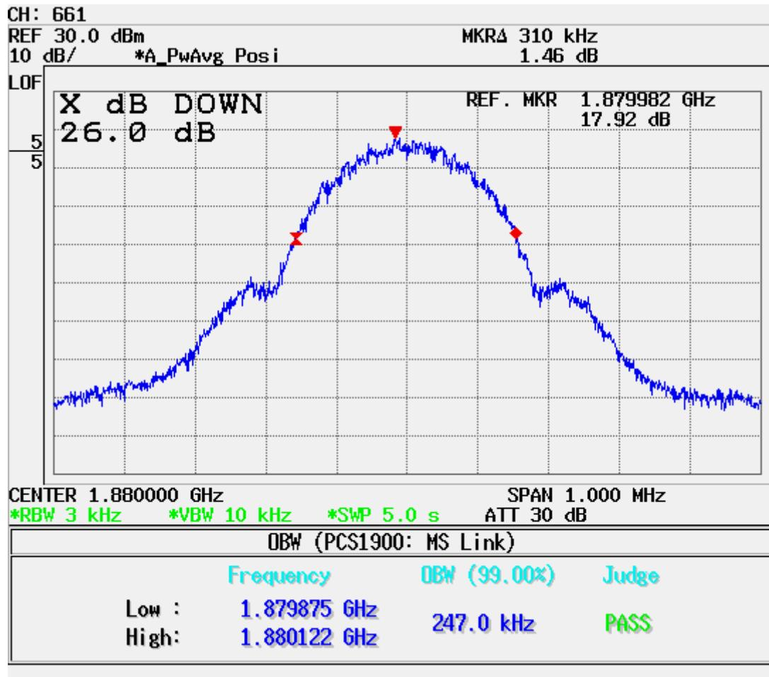
**■ Occupied Bandwidth – 26 dBc BW (KHz) (GSM1900 810 CH)**
