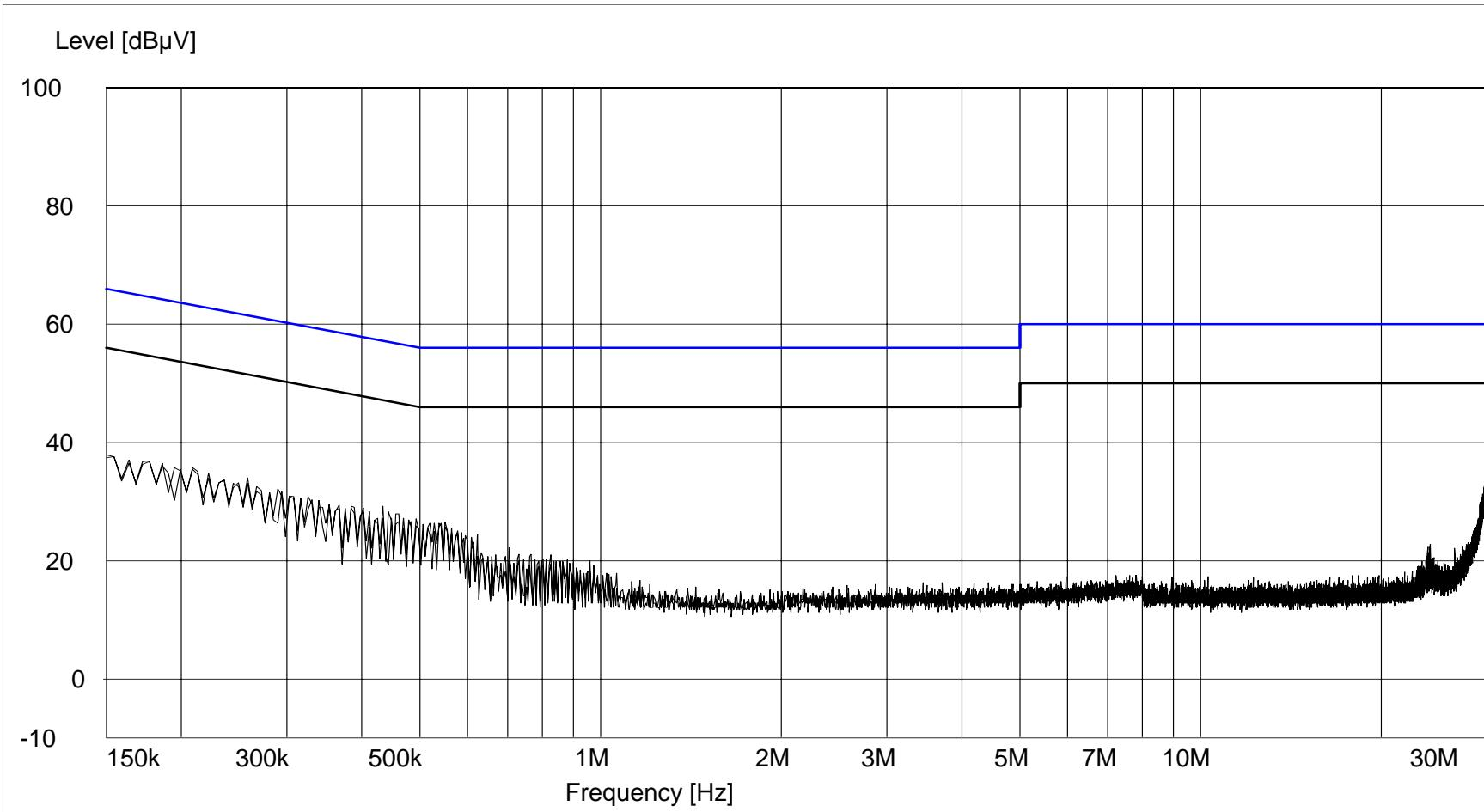
**FCC Part 15, Subpart B, Section 15.107(a), Conducted Emissions, Power Leads,
