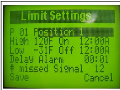
**High** – The High Temperature is the maximum temperature the location of the probe can be before an alarm on the Temp Minder turns on.
