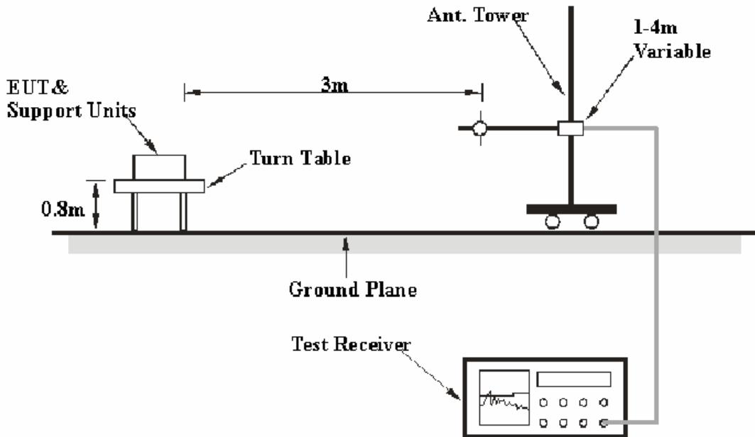
The radiated emission and out of band emission tests were performed in the 3 meters chamber B, using the setup accordance with the ANSI C63.4-2003. The specification used was the FCC 15.209 and FCC 15.249 limits.
