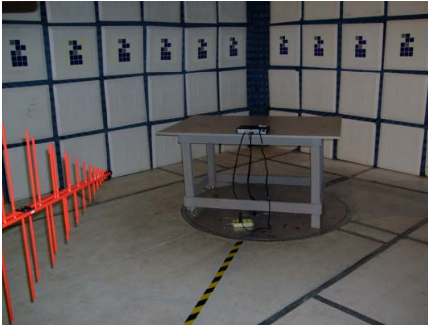
Radiated Emission Test Set-up(Below 1GHz)
