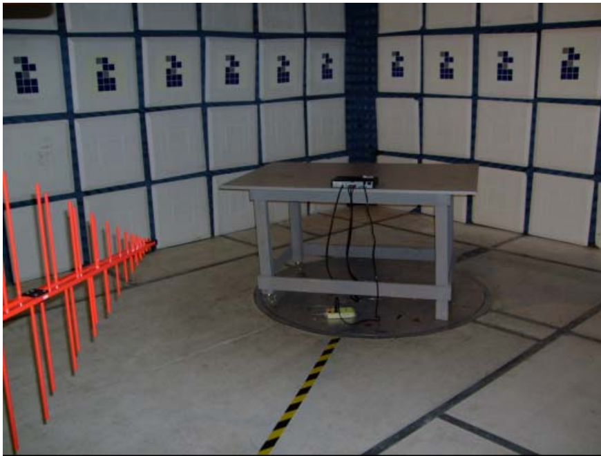
Output and Spurious level test set up photo
