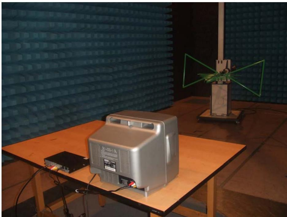
*3. Radiated Emission Measurement(1000-5000MHz)*
