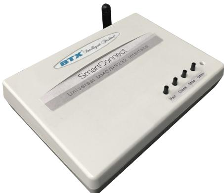
The BTX SmartConnect can be used to communicate between third-party automation systems and BTX's MMC RF motors and controls. The SmartConnect can control units individually or as groups, and is operated via RS232 input. Once the input is executed, a wireless MMC RF radio command is sent to the automated BTX window coverings system.
