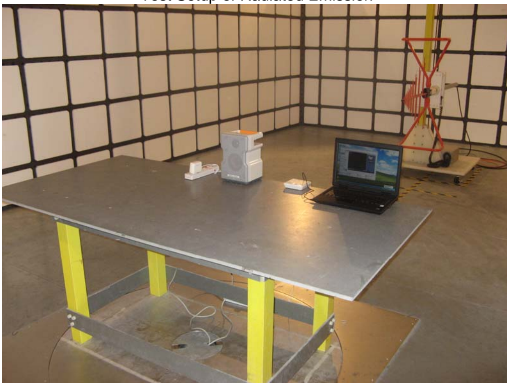
Test Setup of Radiated Emission
