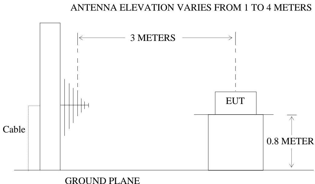
(EUT: Invisible Sliding Wall Vault)
