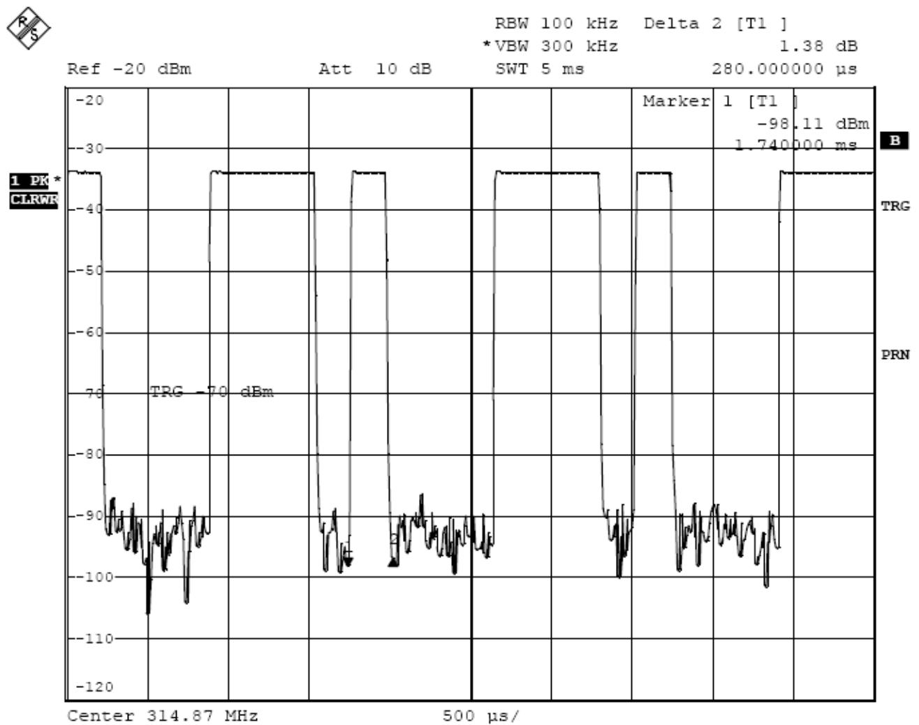
The graph shows the duration of short 'on' signal. From marker 1 to marker 2, duration is 0.28ms.
