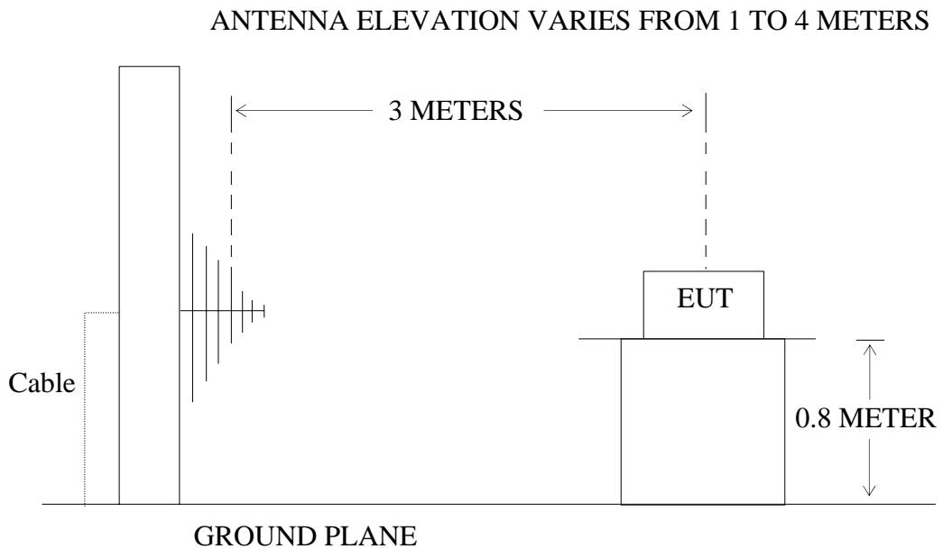
(EUT: Invisible Sliding Wall Vault)
