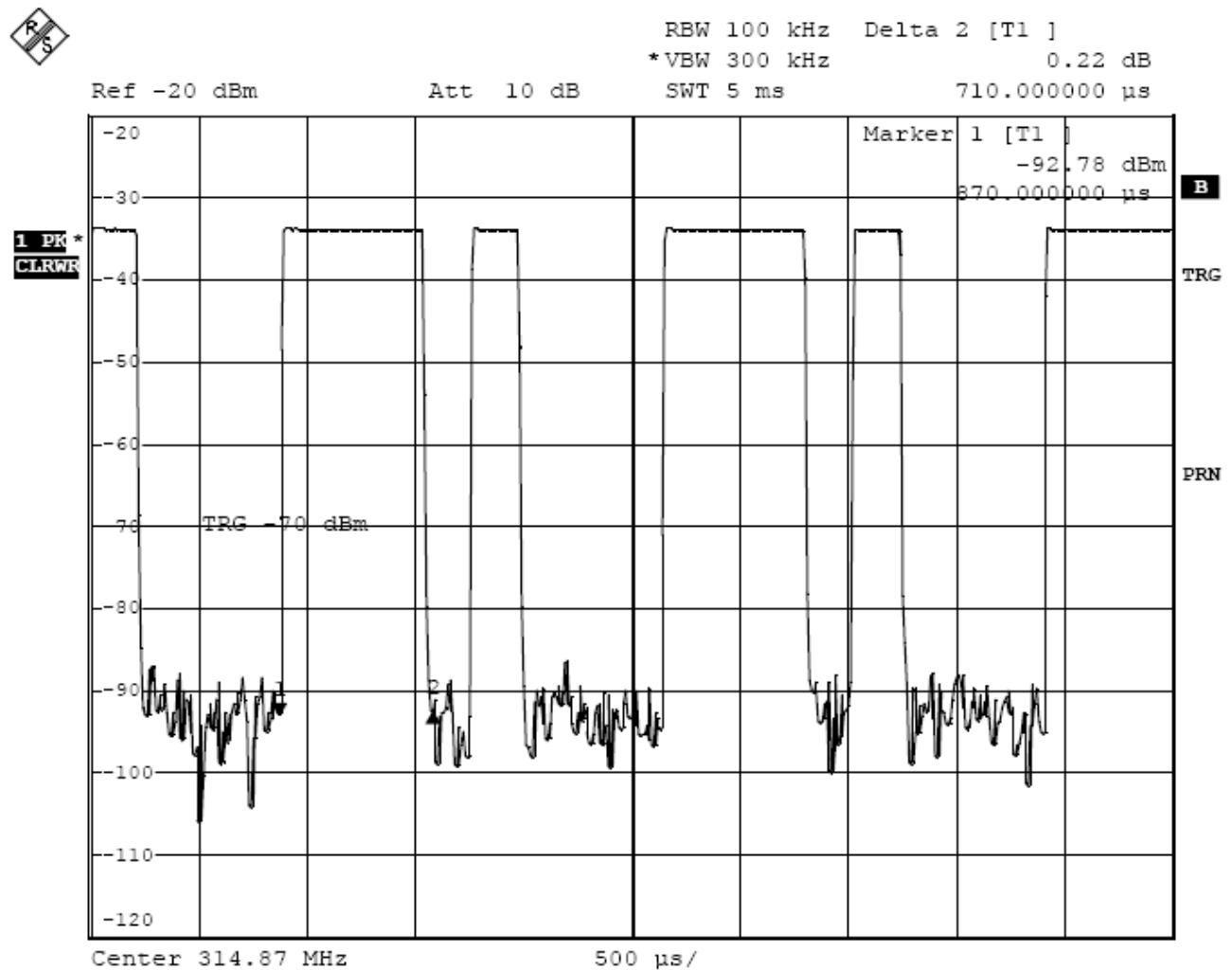
The graph shows the duration of long 'on' signal. From marker 1 to marker 2, duration is 0.71ms.
