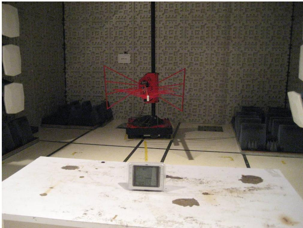
**TEST SETUP OF RADIATED EMISSION (1GHz -2GHz)**
