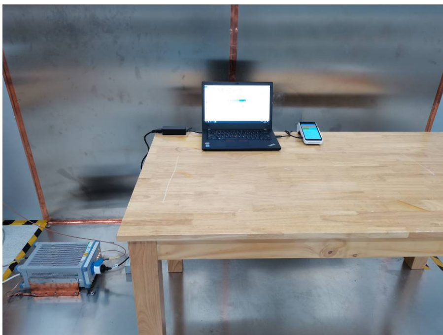
Photograph 1: Set-up for Conducted Emission on AC Mains
