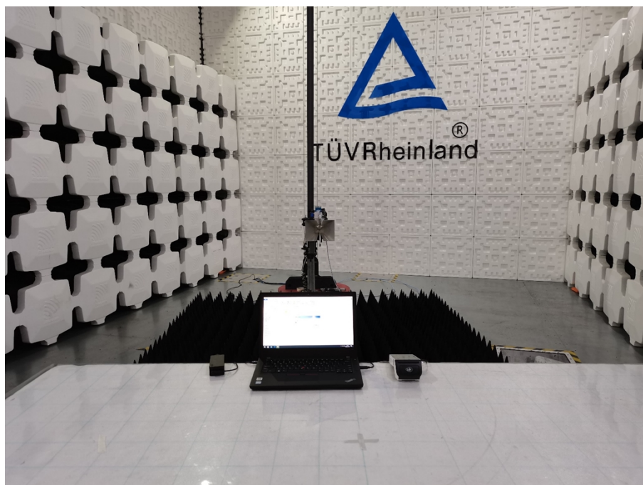
Photograph 3: Set-up photo for Radiated Emission, Above 1GHz
