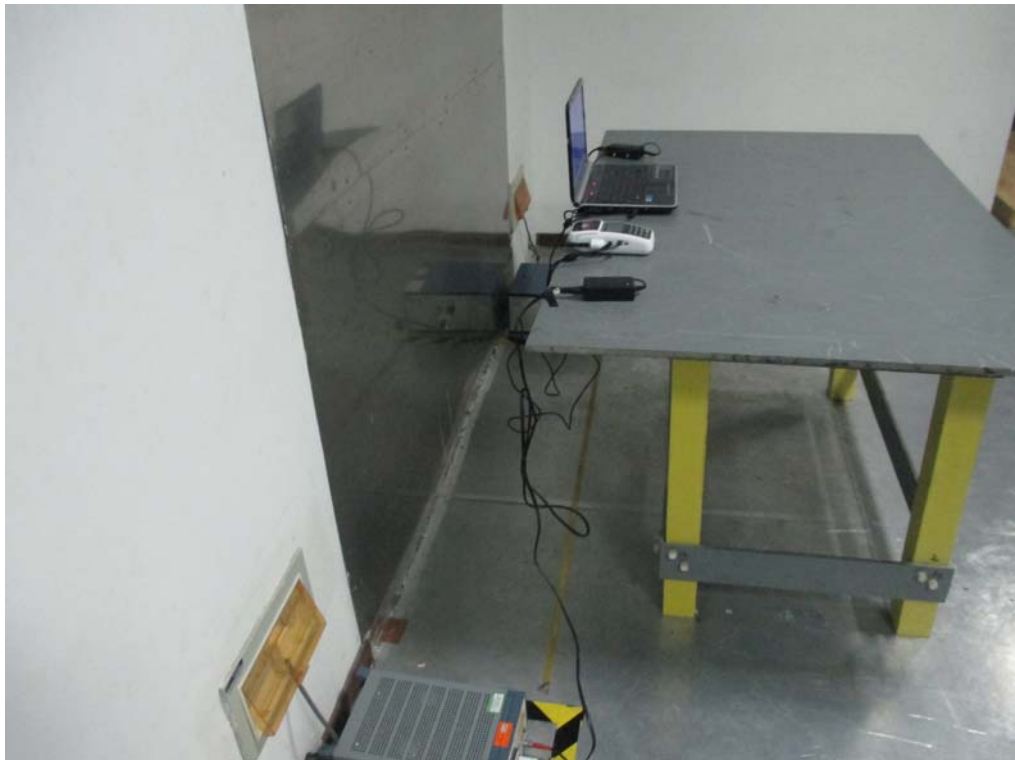
Conducted Emissions Test Setup Side View
