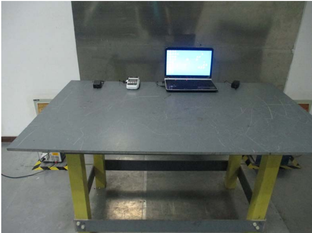
Conducted Emissions Test Setup Front View
