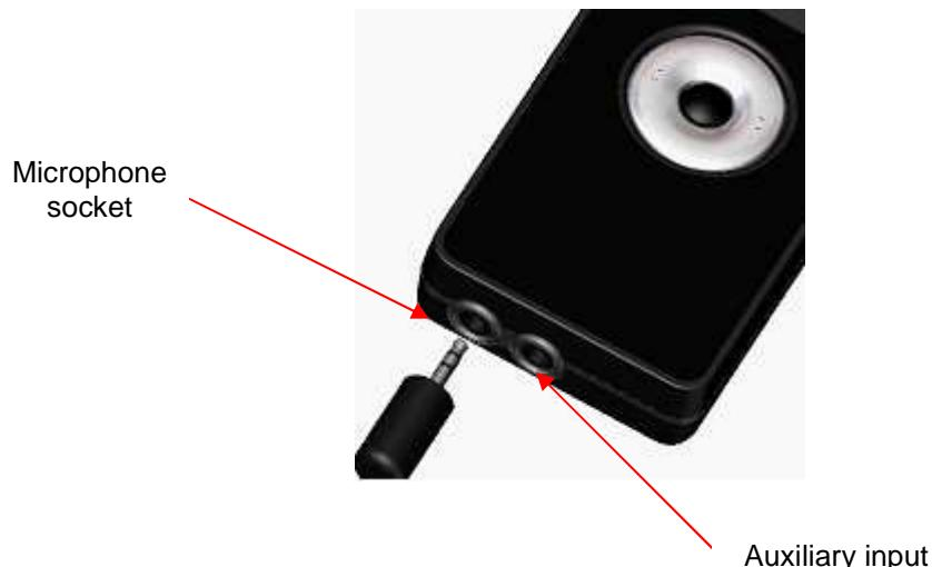
For devices in receiver mode, visitors using headphones can connect one or two earphone(s) (or headphone(s) simultaneously to the dedicated headset (standard jack 3.5 mm).
