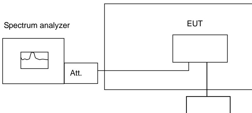
**Remark:** Measurement setup for testing on Antenna connector
