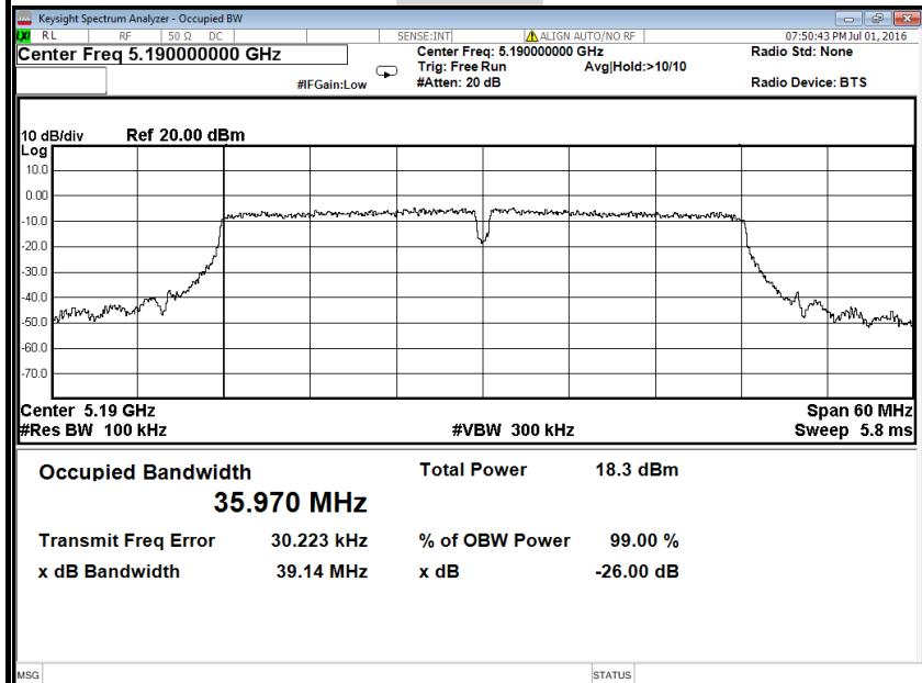
**26dB Bandwidth (CH High)****Antenna 1**
