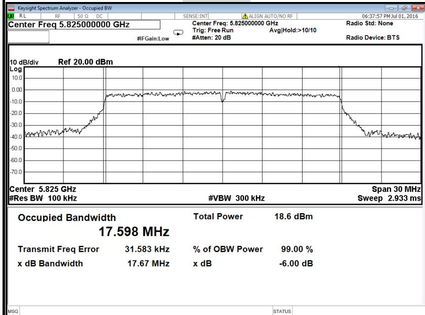
**IEEE 802.11n HT 20 MHz mode / 5745 ~ 5825MHz****6dB Bandwidth (CH Low)****Antenna 1**
