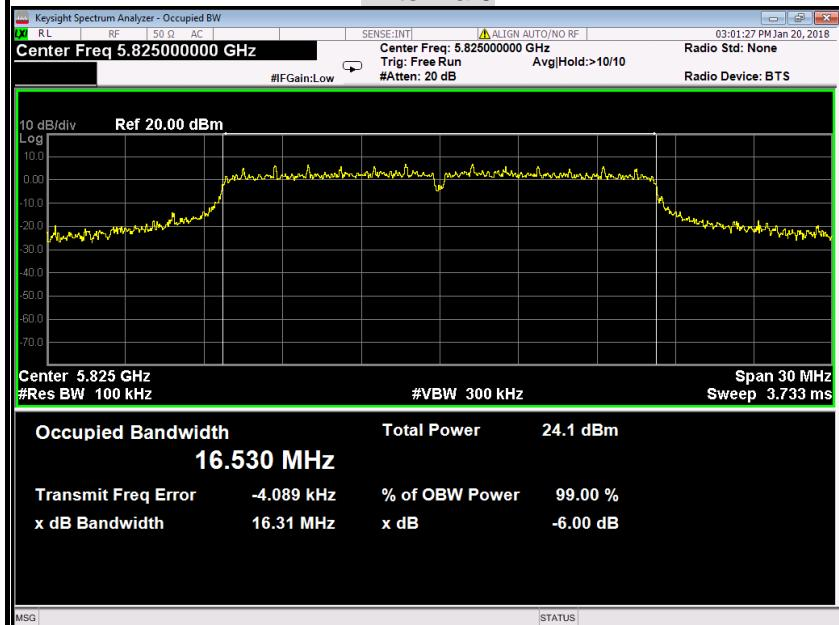
**IEEE 802.11a mode / 5745 ~ 5825MHz****6dB Bandwidth (CH Low)****Antenna 1**
