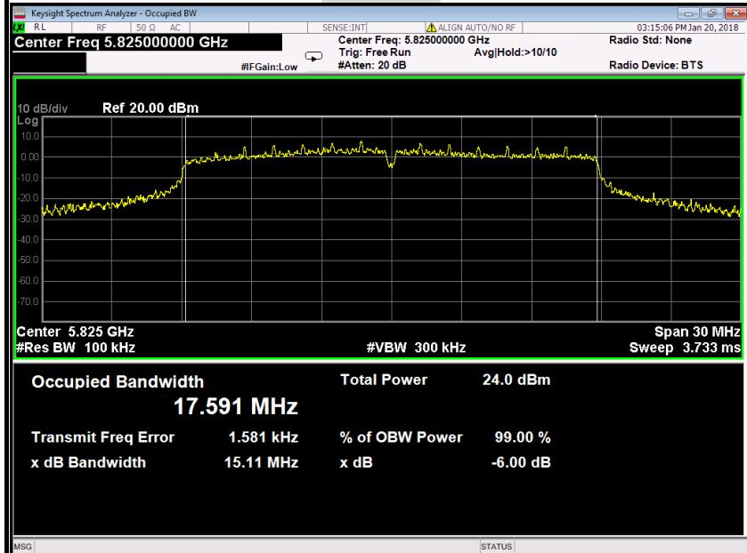
**IEEE 802.11n HT 20 MHz mode / 5745 ~ 5825MHz****6dB Bandwidth (CH Low)****Antenna 1**
