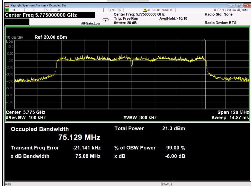
**IEEE 802.11ac 80 MHz mode / 5775MHz****6dB Bandwidth****Antenna 3**
