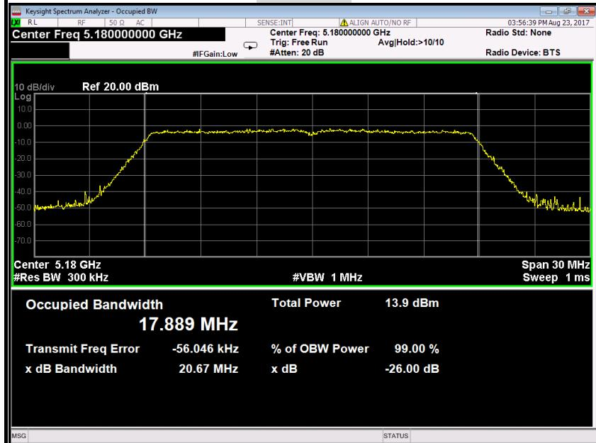
**26dB Bandwidth (CH Mid)****Antenna 0**
