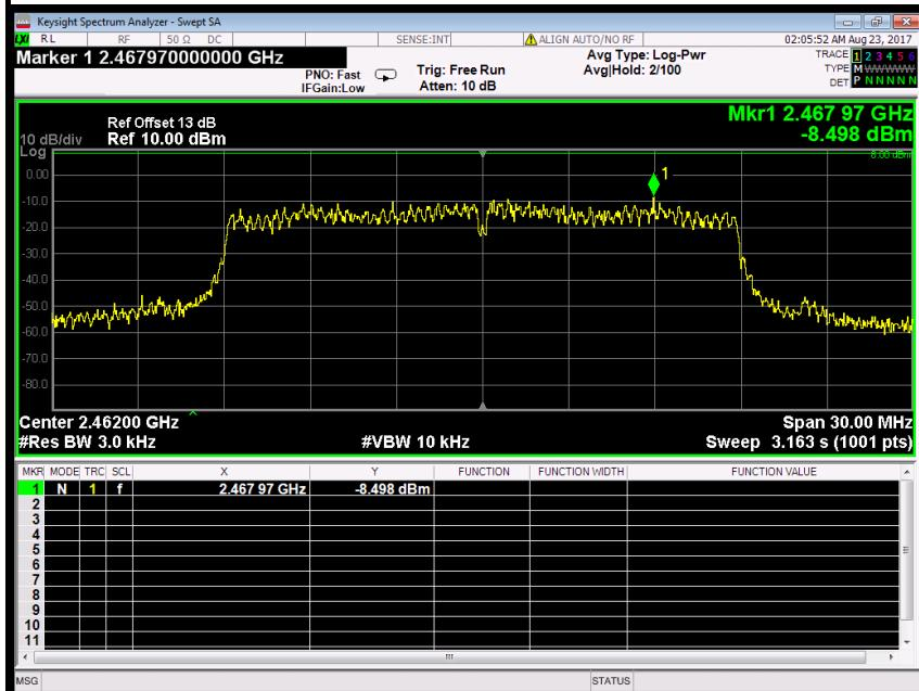
**IEEE 802.11n HT20 MHz mode (Antenna 1)****PPSD (CH Low)**
